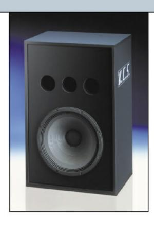
The **C-118-A** houses one K.C.S. S-1846 18" Ø woofer. This is extra-long excursion cone driver featuring 4" Ø coil, massive magnetic circuitry, and carefully engineered cooling schemes, resulting in high power handling and low power compression. The speaker is arranged as a direct radiator, resulting in a deep and highly linear bass sound.
