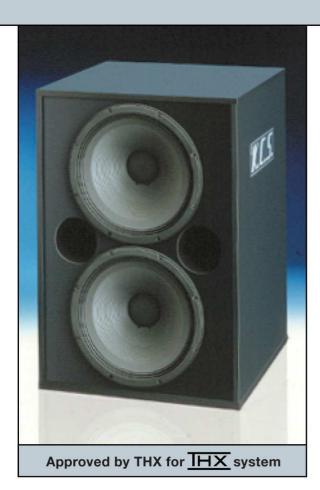
The C-218-A houses two K.C.S. S-1846 18" Ø woofer. These are extra-long excursion cone drivers featuring 4" Ø coils, massive magnetic circuitry, and carefully engineered cooling schemes, resulting in high power handling and low power compression. The two speakers are arranged as direct radiators, resulting in a deep and highly linear bass sound.
