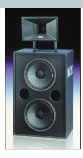
K.C.S. acoustic systems **S-2500** and **S-2501** are a high quality set specially designed as a screen channel group for medium sized cinema theaters. These acoustic systems include a direct radiation technology bass cabinet with twin 15" Ø woofer. The treble system include a compression driver with 4" Ø titanium membrane and 2" Ø mouth with constant directivity horn.
